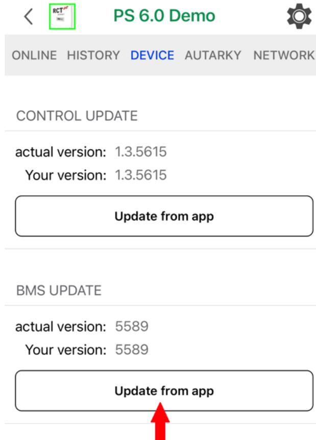
After the successful update, the battery master will update every battery module independently to ensure identical software versions and the system won't be able to use the batteries for a short time. You can see the update process by the red-green flashing LED on the bottom of the BMS.
