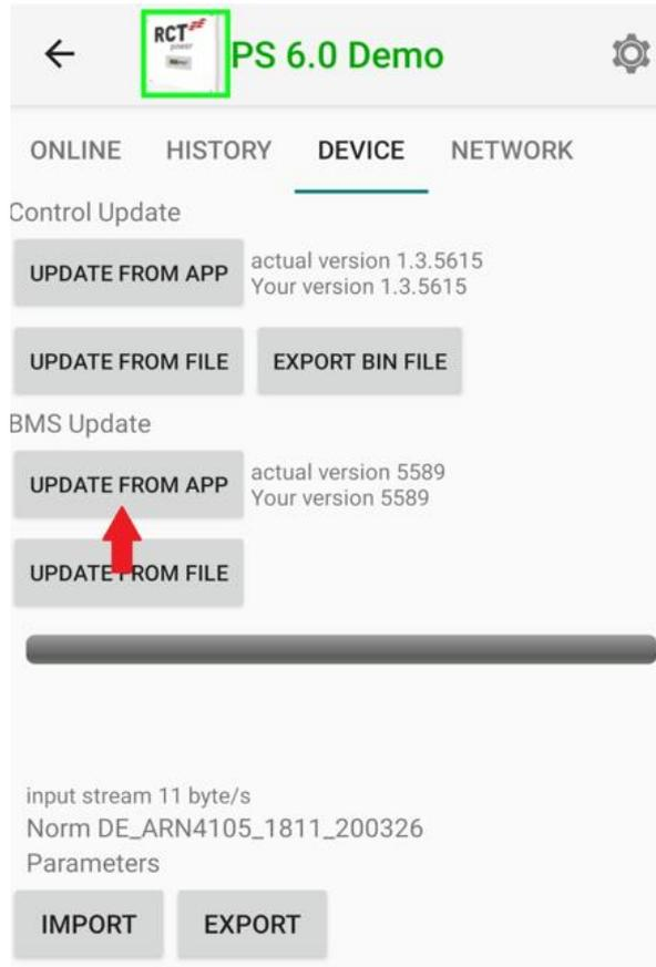
After the successful update, the battery master will update every battery module independently to ensure identical software versions and the system won't be able to use the batteries for a short time. You can see the update process by the red-green flashing LED on the bottom of the BMS.
