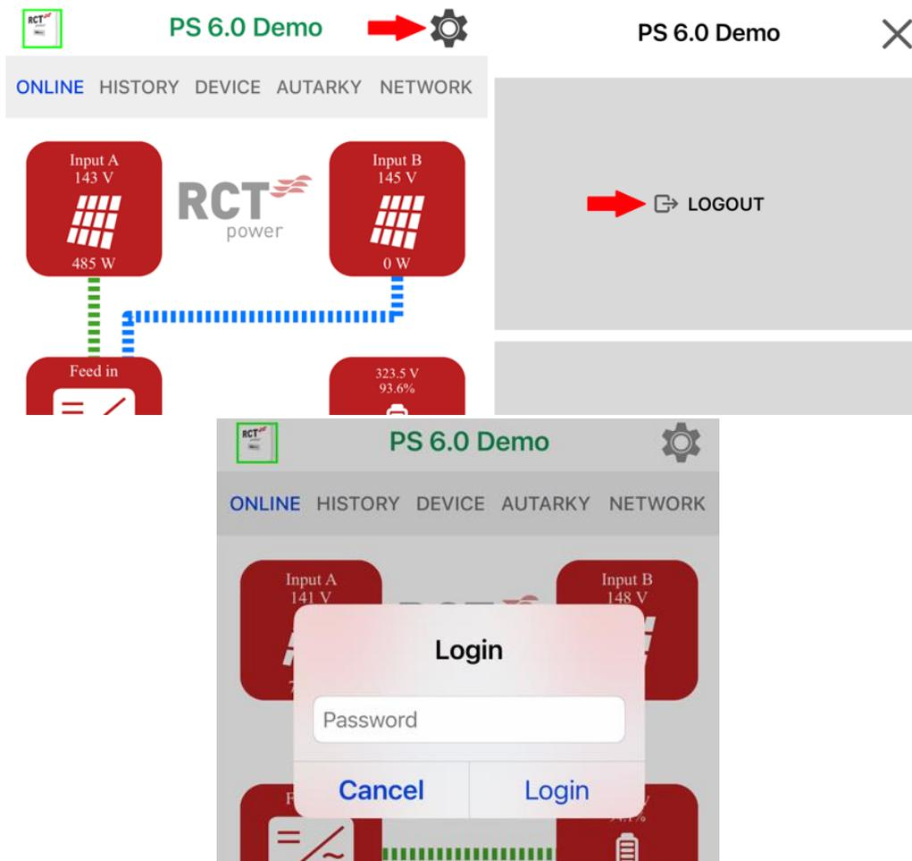
Now tap back (e.g., with the arrow at the top left corner) and navigate to the needed menu with "device" → "settings" → "update":
